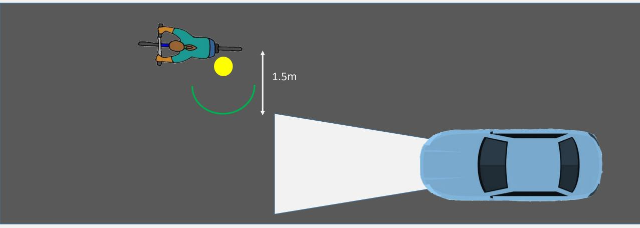
Car driver recognises the required distance as a projection on the road LEDs show the width of the bi-cycle
