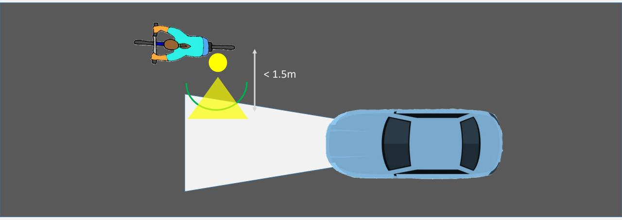
Additional warning LEDs switch on when the vehicle falls below a horizontal distance of 1.5 m In addition the bi-cycle driver is brightly illuminated from below
